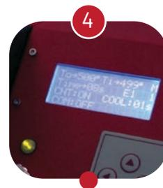
The pre-programming of references can be done manually or using a PC with STCS-RCT software (reads Excel™ files)
