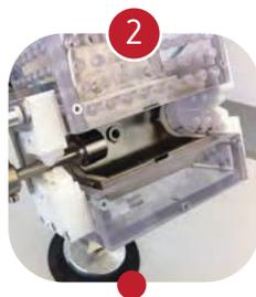
Can be supplied with customized clamps with automatic holding system, cooling system or end splice tool
