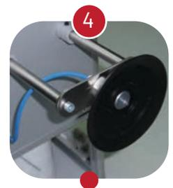
Holding to the panel using a suction vacuum pump, which can be positioned horizontally or vertically
