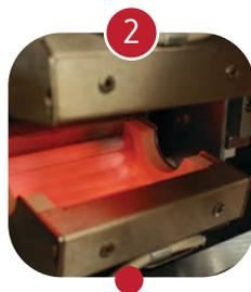
Quartz infrared oven that allows higher temperatures
