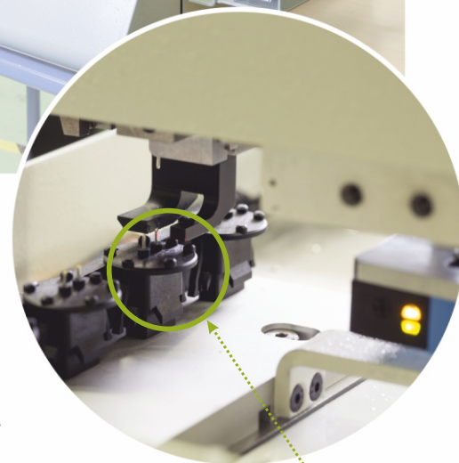
Alignment supports for plastic components
