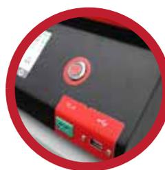
USB and Ethernet sockets for network communication
